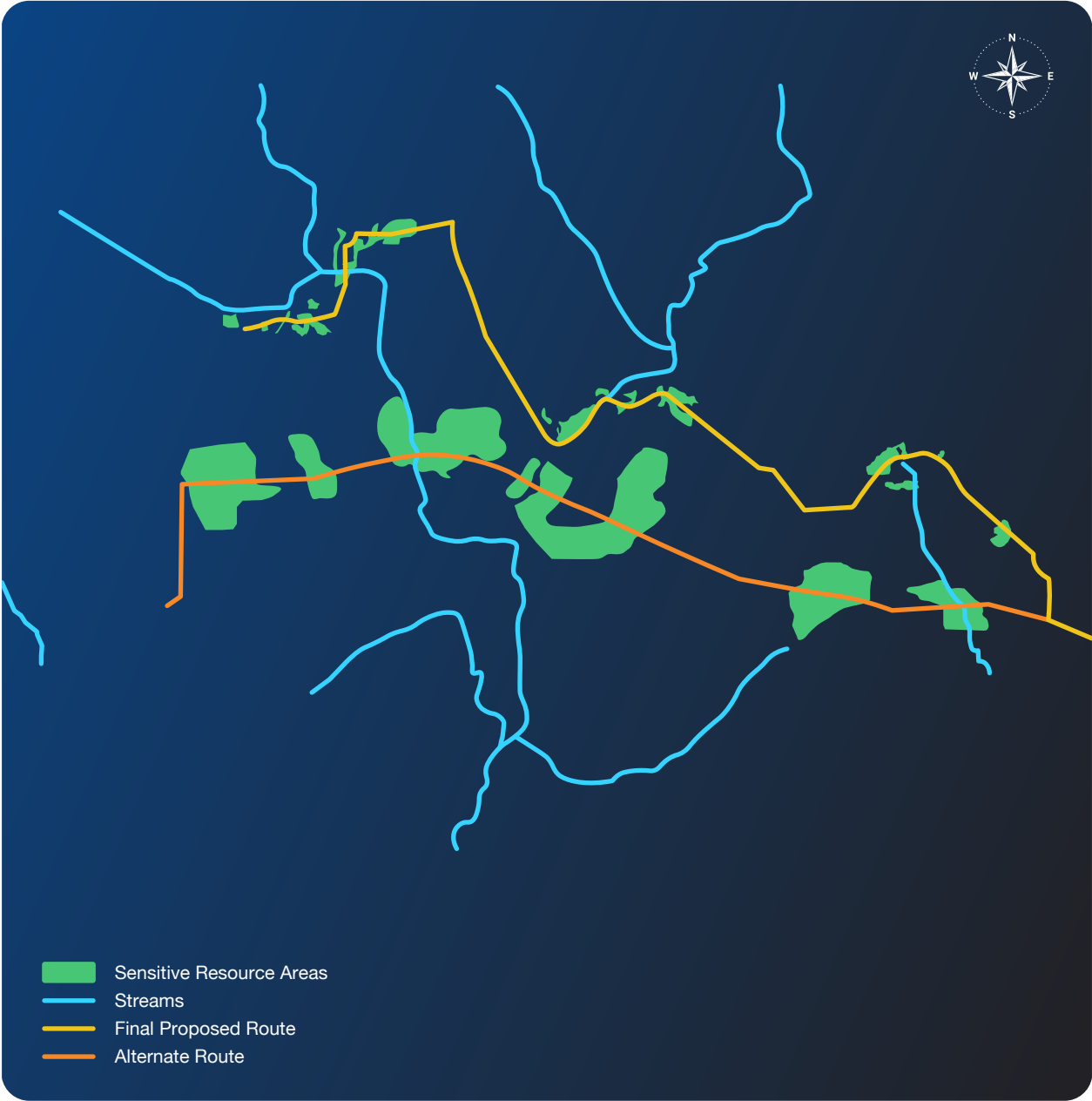
For all pipeline expansion projects, Williams evaluates impacts to sensitive resource areas alongside the planned route and multiple alternate routes. In this example from the Housenick Pipeline, the final proposed route crossed some streams, but still had much less overall impact to high-value sensitive resource areas, such as wetlands and forested areas, than the alternate route.
