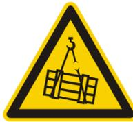
Contractor shall ensure a safe distance shall be maintained when a load is suspended in the air.
