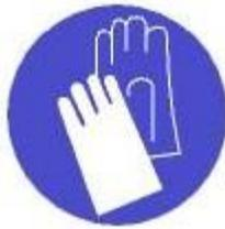
Appropriate gloves (cloth, cut-resistant, leather or leather-palmed gloves) must be worn when hands are exposed to potential hazards such as burns, cuts, punctures, or abrasions, when handling chemicals or hazardous materials where absorption is a concern (chemical resistant gloves), and when performing electrical work (certified gloves for electrical work).
